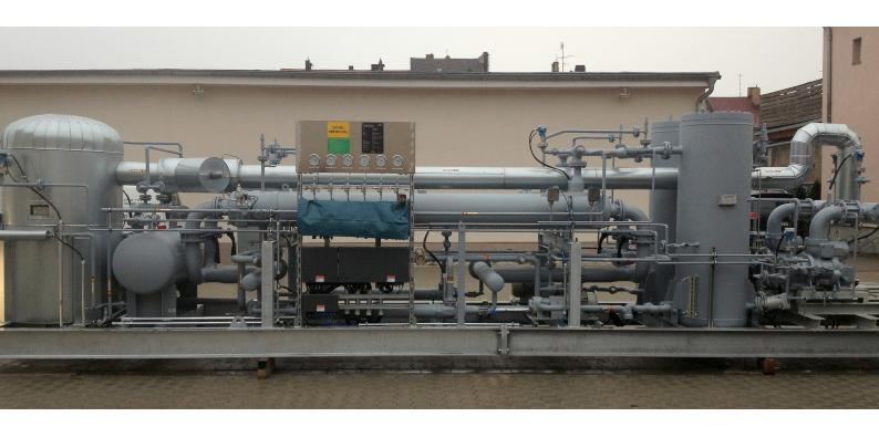
Polar Refrigeration delivered a screw compressor skid to a chemical plant where major part is production of ammonia (NH3).
